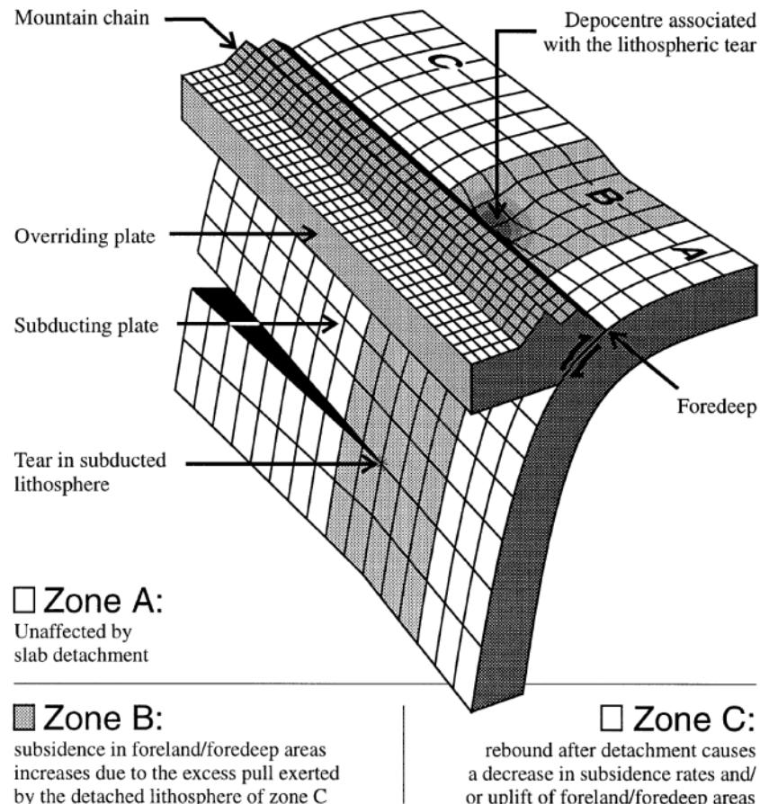
Fig. 1. Graphical representation of the hypothesis of lateral migration of slab detachment (Wortel and Spakman, 1992), and predicted surface effects. Reprinted from van der Meulen et al. (1998) with kind permission of Elsevier Science.
