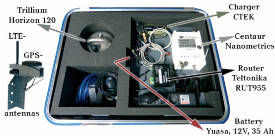
Figure 2: DSEBRA station equipment.
